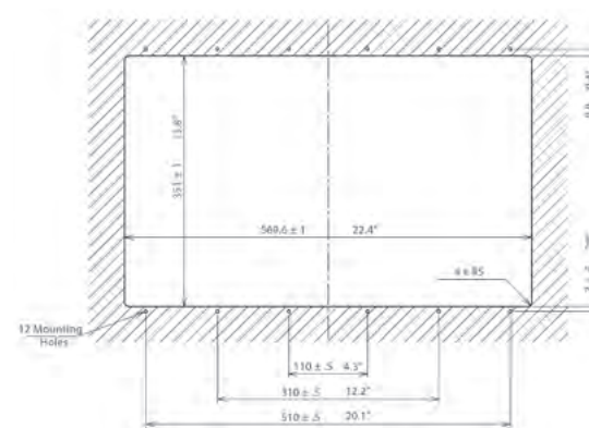
Multi Function Display Flush Mount TZT24X Cutout Dimension
